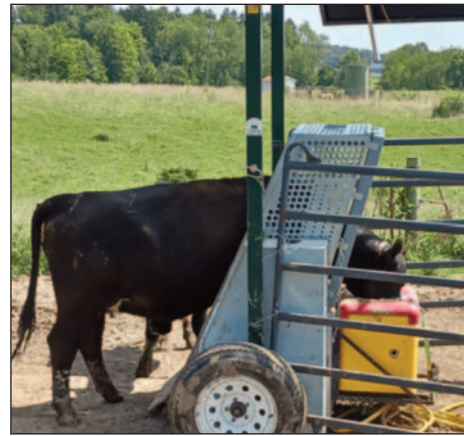
Figure 1: Mobile Vytelle SENSE (TM) weigh system with water as attractant used to record animal weight and water intake.
