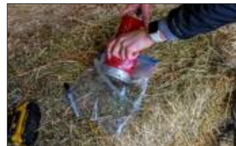
Figure 4. Always submit the entire sample. Subdividing the sample can result in altered lab results since the fine material segregates from the larger particles. Make sure the bag is clearly labeled with all required information.
